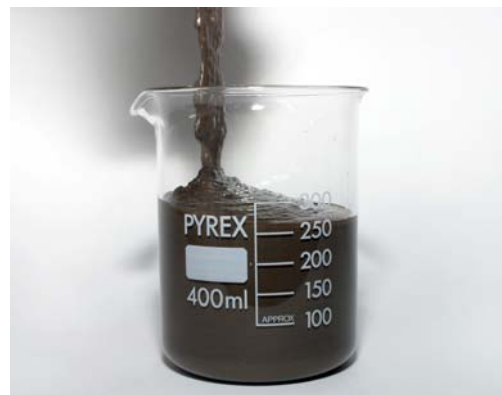
North Sea shale cuttings slurrified using 2.5%wt SAS ME product and 2.5%wt sea water assume free flowing fluid characteristics similar to OBM.
