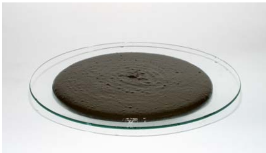
North Sea shale cuttings slurrified using 2.5%wt SAS ME product and 2.5%wt sea water. Notice the enhanced fluidised nature of the waste.
