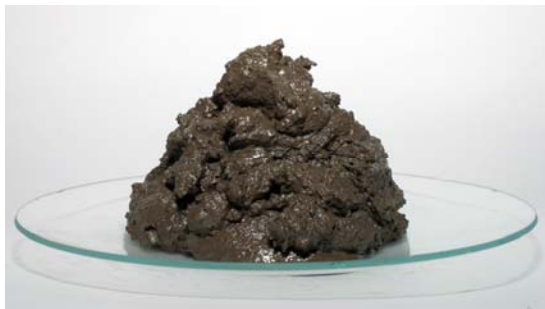
North Sea shale cuttings slurrified with 50%wt sea water under low / no shear mixing conditions.
