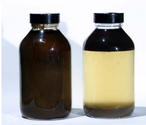
Wellbore cleanup waste slop before and after the split using SAS microemulsion product.
