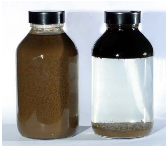
Mud pit cleaning waste slop before and after the split using SAS microemulsion product
