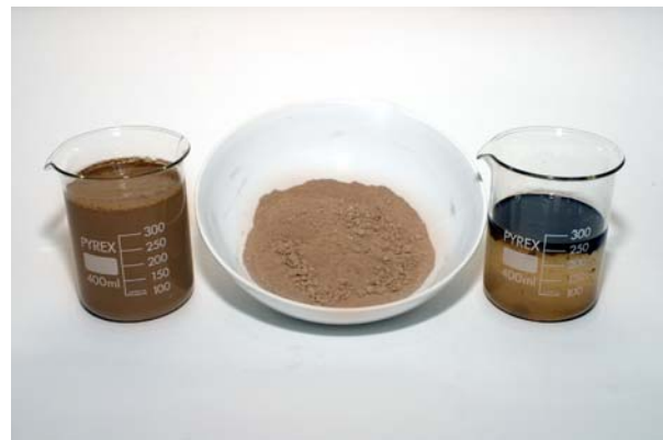
Tank bottom slops split into clean solids, water and recovered oil fractions using SAS microemulsion product
